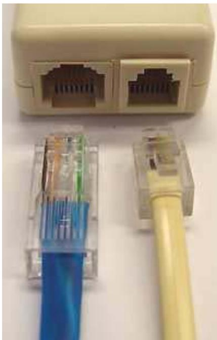
On the right is an RJ-11 socket (also called RJ-12) and a telephone cable with an RJ-11 plug on the end that will allow it to fit into the socket.
